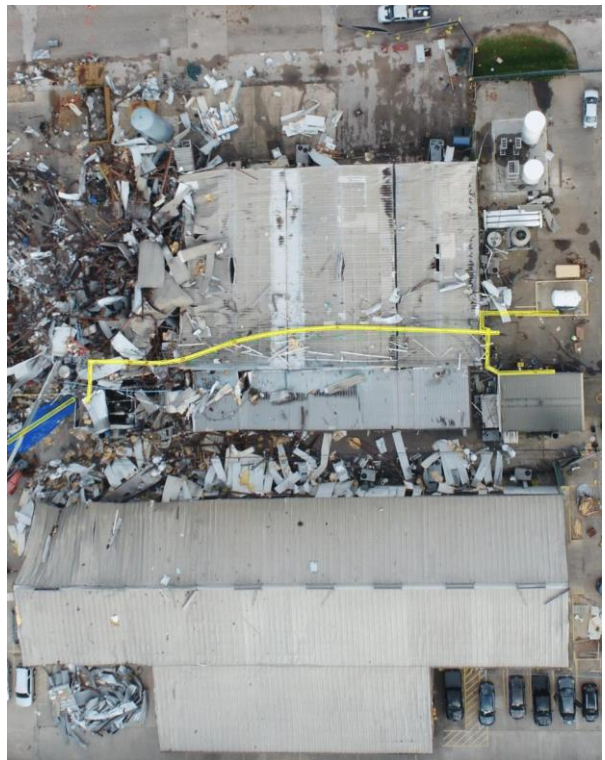
Pre and Post explosion aerial photos of Coating building (left) and ball lapping building/machine shop (right) with Propylene pipe remains highlighted in yellow. (Propylene piping denoted in the Pre-incident photo in red)
