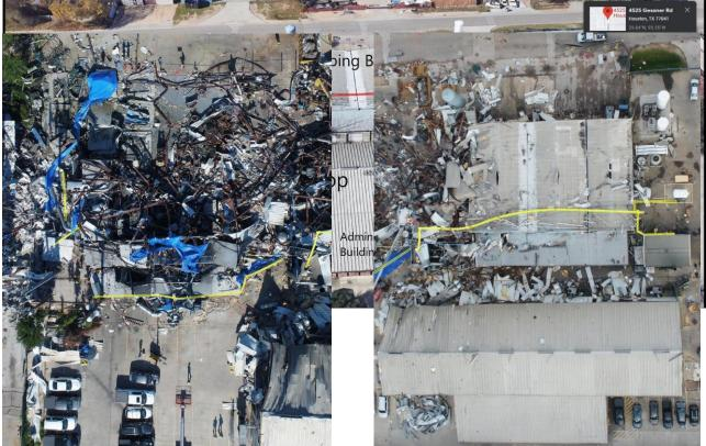
Pre and Post explosion aerial photos of Coating building (left) and ball lapping building/machine shop (right) withPropylene pipe remains highlighted in yellow. (Propylene piping denoted in the Pre-incident photo in red)
